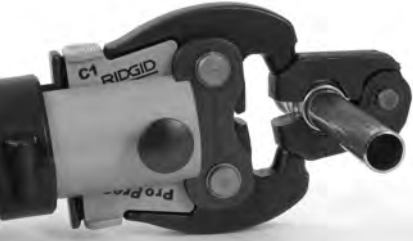
Figure 10 – Attaching Actuator to Press Ring
