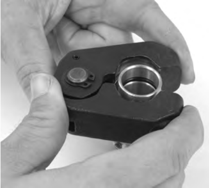
Figure 9 – Installing Press Ring onto Fitting
