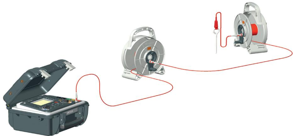
Plug the lead from one cable reel into the centre of the next cable reel, to form a daisy chain of cable reels, to extend usable range. Use the provided lead (with a crocodile clip) to connect from the centre plug of the cable reel to a spike in the ground.
