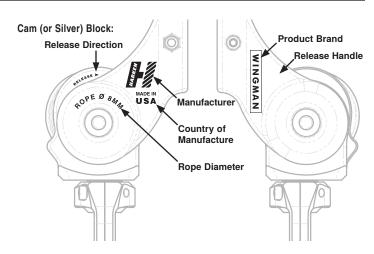
open the release handle and release it. Verify the release handle snaps closed. Pull on the haul/tail end of the rope and verify the sheaves turn freely and you hear a clicking sound.
